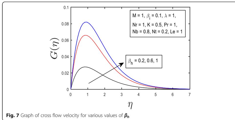
**Fig. 7** Graph of cross flow velocity for various values of  $\beta_h$
