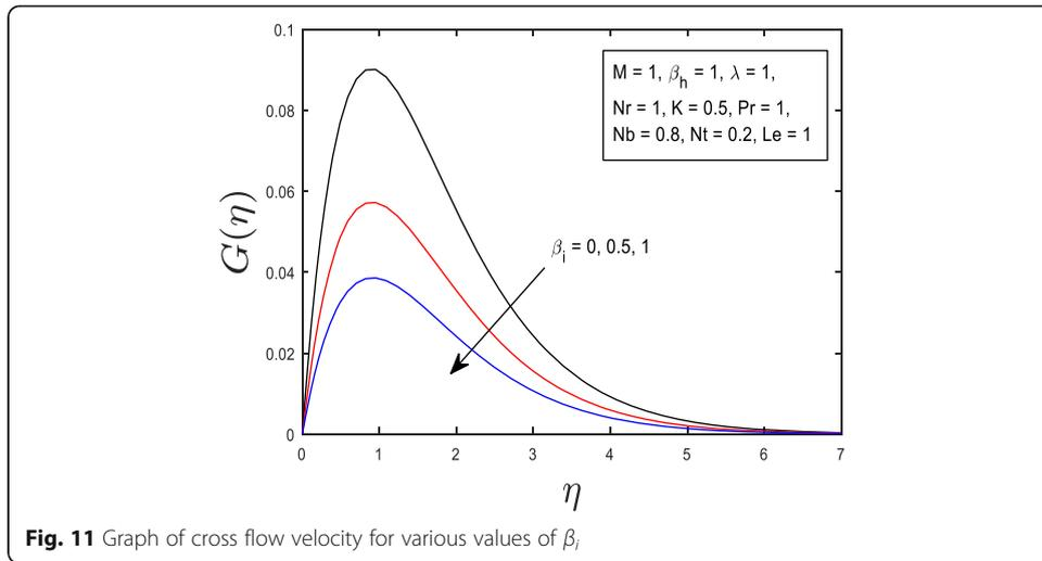
**Fig. 11** Graph of cross flow velocity for various values of  $\beta_1$
