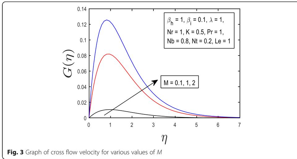
**Fig. 3** Graph of cross flow velocity for various values of  $M$
