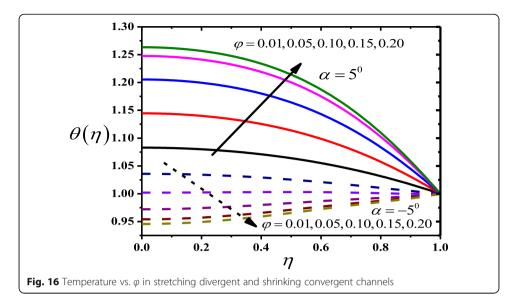
enhances extensively. Also, Table 3 confirms that heat transfer rate considerably enhanced as estimation of volumetric parameter increases. However, the shrinking convergent channel shows contrary behavior for same condition. In other words, the thermal boundary layer decreases on enhancing the value of  $\phi$  in shrinking/convergent channel.
