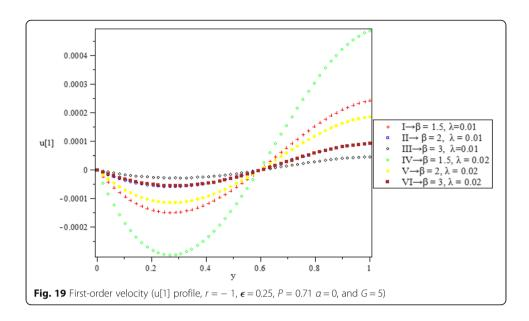
difference in the flow, which enhances fluid velocity. Also when there is heat sink (i.e.,  $\alpha$  < 0), the velocity decreases with an increase in Grashof number (G) (see curves I and IV).
