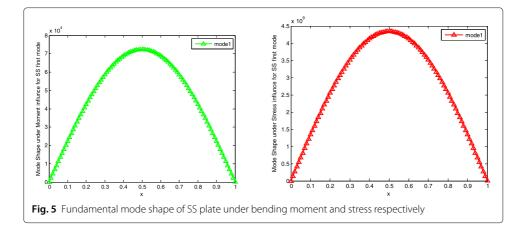
the vibrating plate changes. While Fig. 6 depicts the extrema mode shape variation. It is clearly revealed that Figs. 5 and 6 when compared to Fig. 4 have different mode shapes. Invariably, the extrema mode shape location differs based on the boundary conditions. When the plate is submerged in fluid, the same mode shapes as illustrated in Fig. 4 are obtained; this is in accordance with the experimental result obtained by [33, 34]
