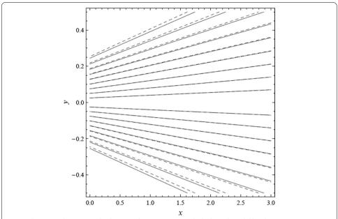
**Fig. 5** The stream line y is graphed against the parameters x which show the solid line by (Re = -5, m = 0:3) and dotted line by (Re = 5, m = 0:3)
