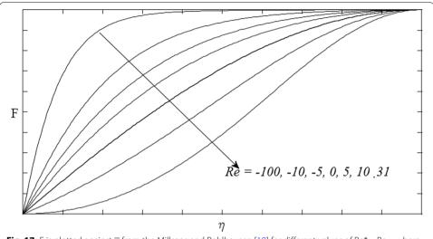
**Fig. 17** F is plotted against  $\overline{\eta}$  from the Millsaps and Pohlhausen [18] for different values of Re\*=Re $\alpha$ , where  $\alpha$  is the inclination angle of the channel
