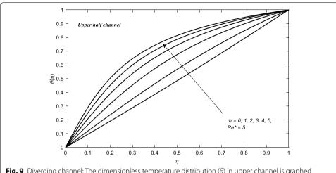
**Fig. 9** Diverging channel: The dimensionless temperature distribution ( $\theta$ ) in upper channel is graphed against  $\eta$  for  $c_1 = 0.1$  and Pr = 1
