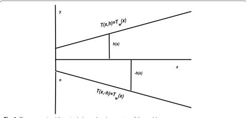
Fig. 1 The converging (diverging) channel and geometry of the problem
